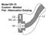
**Figure 3-4:** The ER-15 earplug uses a combination of cavities, resistances, and volumes to yield a flat (or unchanged) response at the musicians' ear, but with a 15 decibel attenuation. Picture courtesy of Etymotic Research.
